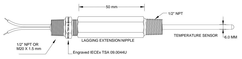
SUITABLE FOR USE WITH CERTIFIED Ex d / Ex e ENCLOSURE OR TRANSMITTER HOUSING WHICH HAS 1/2" NPT OR M20 X 1.5 MM PROCESS CONNECTION
